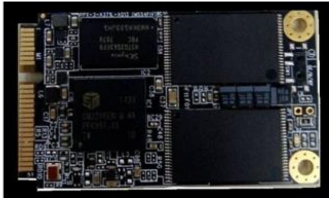
Figure 1: mSATA SSD Overview Diagram
